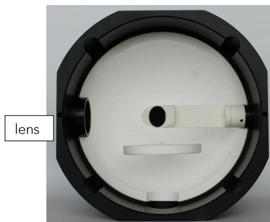
Figure 10. View into the upper half of the sphere; setup for solid samples measurements
