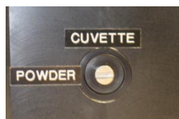
Figure 9. Two position mirror dial set for solid samples measurements
