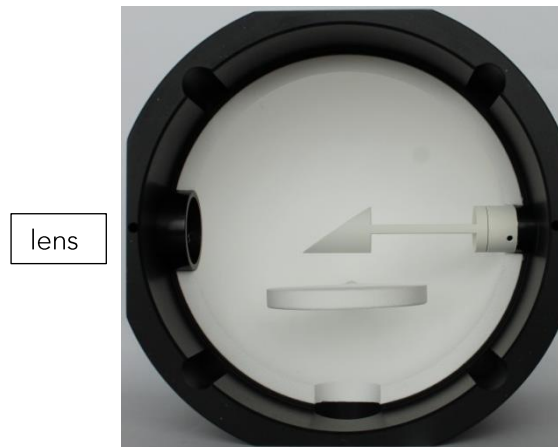
Figure 7. View into the upper half of the sphere; setup for liquid samples measurements
