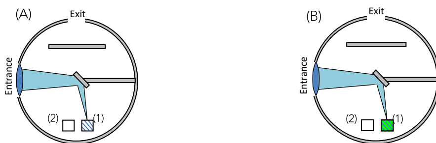
Figure 11. Two different measurement configurations required for Direct APLQY measurements: (A) reference sample (solvent only) in sample position (1); (B) test sample in position 1 (position 2 remains empty for both measurements.)
