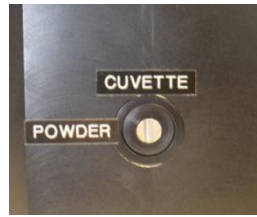
Figure 6. Two position mirror dial set for liquid samples measurements
